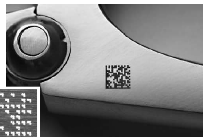
Examples of dot-peening (left), and laser-marking techniques (above).
